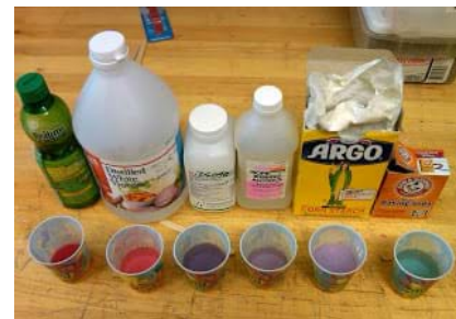
Red cabbage juice changes color to indicate the pH of various everyday items.
